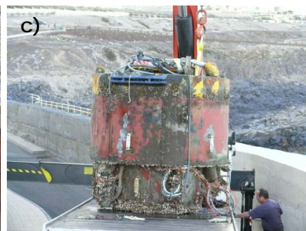
a) Thanos Gkritzalis (NOC sensors engineer) at the PAP Observatory. b) In June 2010 a collaboration between the UK Met Office and NERC led to the deployment of a new mooring at the PAP-SO with an ODAS buoy and full suite of meteorology sensors to complement the existing ocean variables. c) The ESTOC buoy after recovery.
