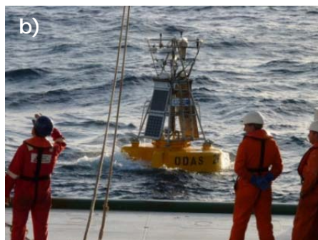
a) Thanos Gkritzalis (NOC sensors engineer) at the PAP Observatory. b) In June 2010 a collaboration between the UK Met Office and NERC led to the deployment of a new mooring at the PAP-SO with an ODAS buoy and full suite of meteorology sensors to complement the existing ocean variables. c) The ESTOC buoy after recovery.
