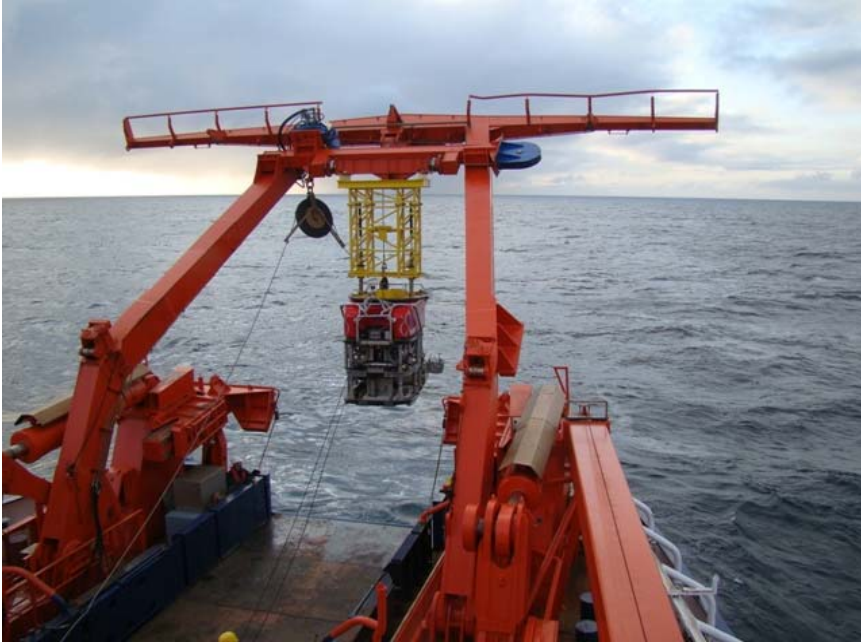
Deployment of the ROV QUEST using the A-frame. Photo: D. Olonschek, AWI
