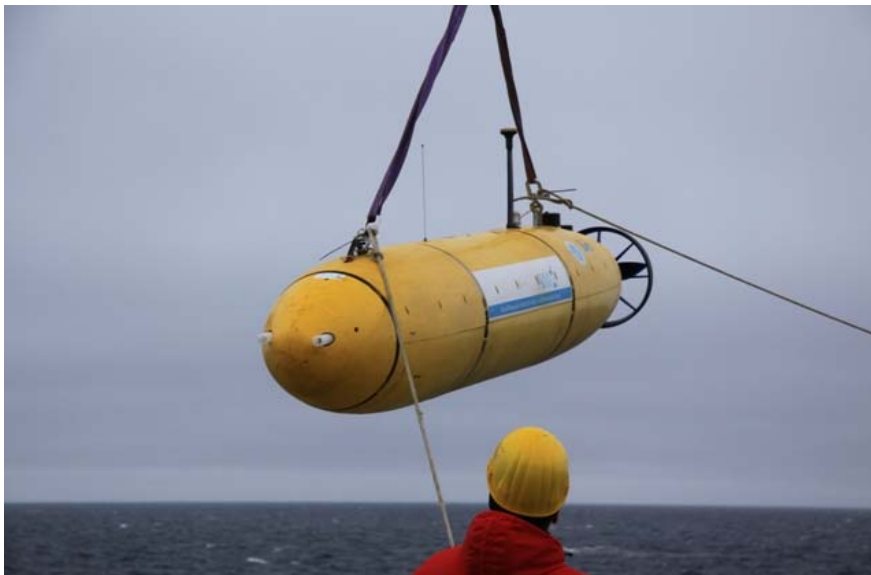
The deployment of the Autonomous Underwater Vehicle is supported by the ship crew keeping the ropes tight. Photo: D. Olonschek, AWI
